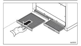
■ Pull the filters out of the slots in the front of the cooker hood housing.
